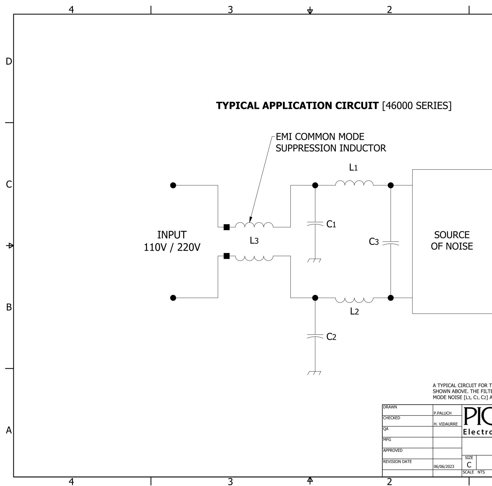
A TYPICAL CIRCUIT FOR THE ELIMINATION OF NOISE IS SHOWN ABOVE. THE FILTER CONTAINS TWO STAGES; ONE FOR COMMON MODE NOISE [L3, C1, C2] AND ONE FOR CONDUCED NOISE [L1, L2, C3]
